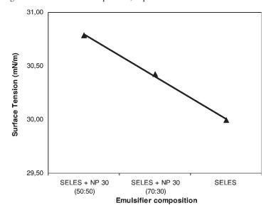
Figure 3. Surface tension of copolymer latexes as a function of anionic emulsifier concentration: SELES + NP30 = 50:50 (% wt), SELES + NP30 = 70:30 (%wt), and 100% SELES.
