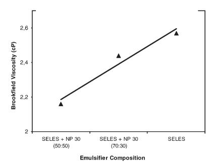
**Figure 1.** Brookfield viscosity of copolymer latexes as a function of anionic emulsifier concentration: SELES + NP30 = 50:50 (% wt), SELES + NP30 = 70:30 (%wt), and 100% SELES.
