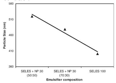
Figure 2. Particle size of copolymer latexes as a function of anionic emulsifier concentration: SELES + NP30 = 50.50 (% wt), SELES + NP30 = 70.30 (%wt), and 100% SELES.
